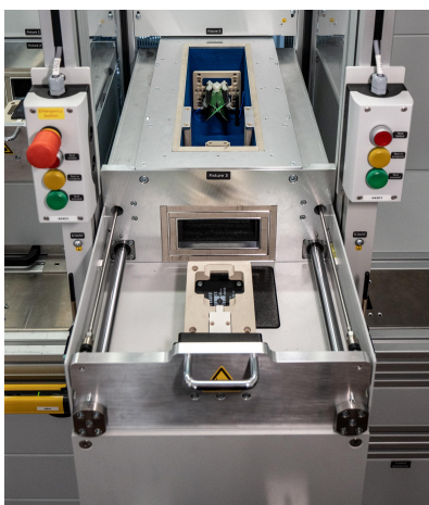
Fixture with open drawer and removed service cover
